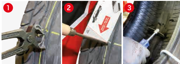
1 Locate and mark the damage. Take or screw out the foreign object. 2 *Determine the direction of the puncture channel. 3 Clean the repair area using LIQUID BUFFER and a scraper.
